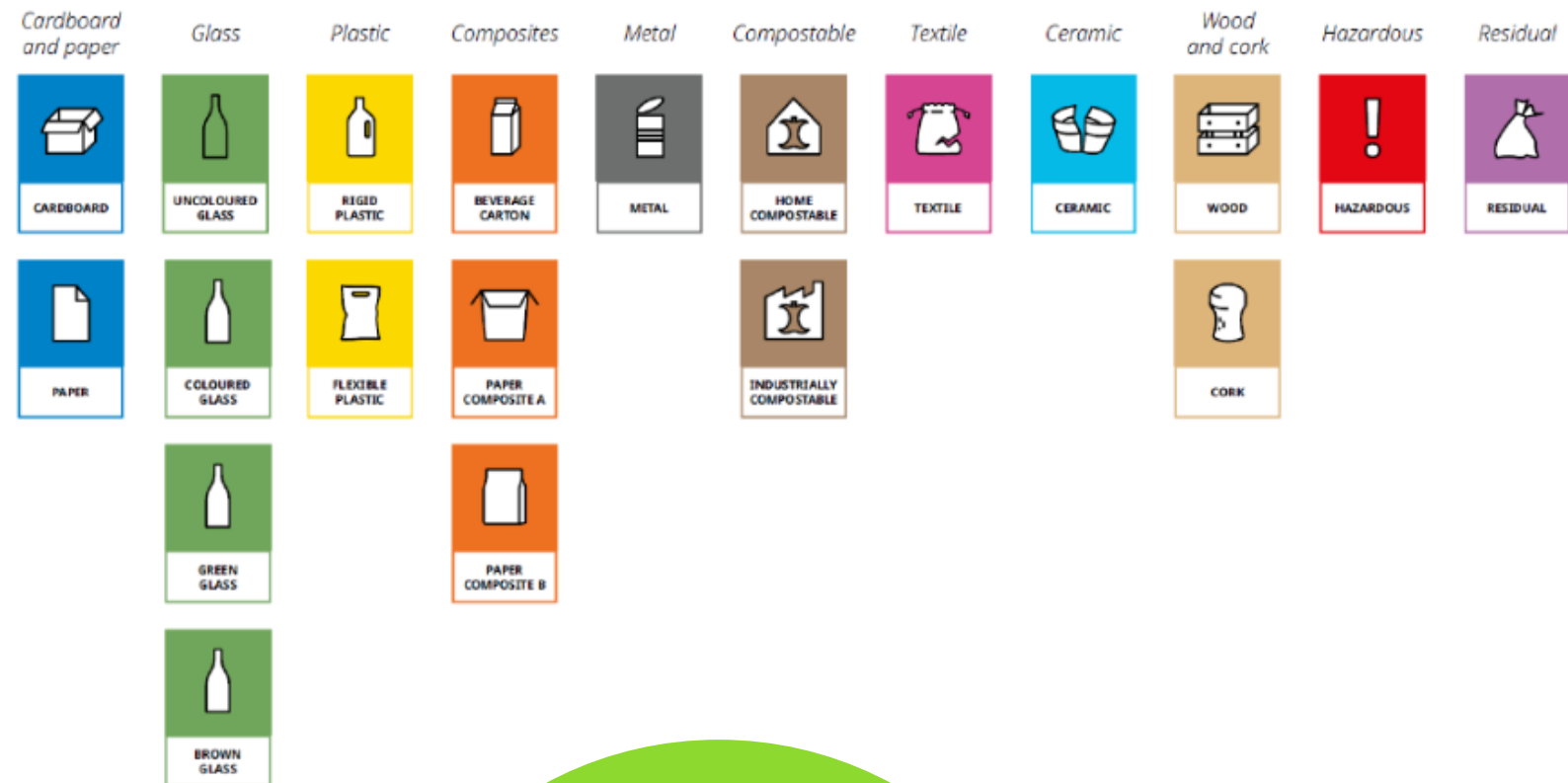
Figure 13. Pictograms and materials as used in the proposed EU harmonised waste sorting labelling scheme.
